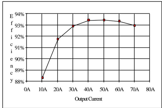
Fig 9. Efficiency versus output current at 54VDC out, 240VAC in.
