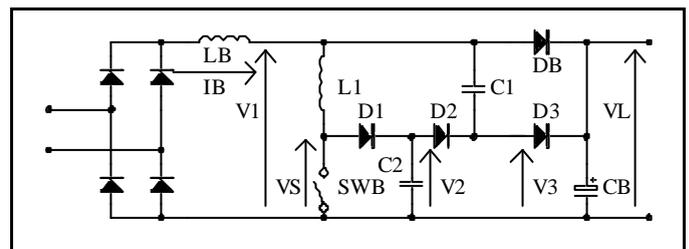
Fig 6. Boost circuit incorporating the new snubber.
