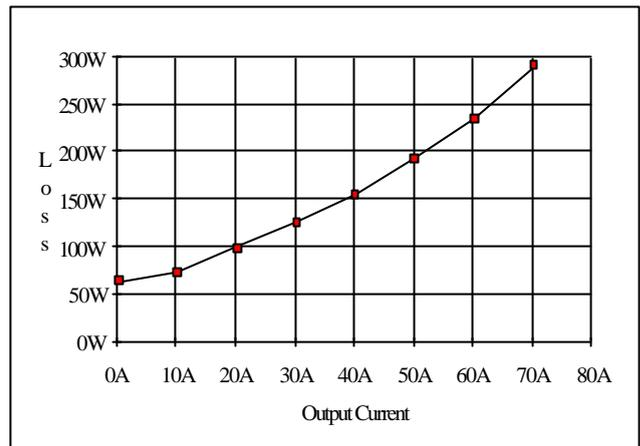
Fig 10 Power loss versus output current at 54V out, 240VAC in.
