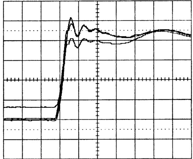
Fig 13. Observed lossless snubber operation at turn-off. 100V/div, 200nsec/div
