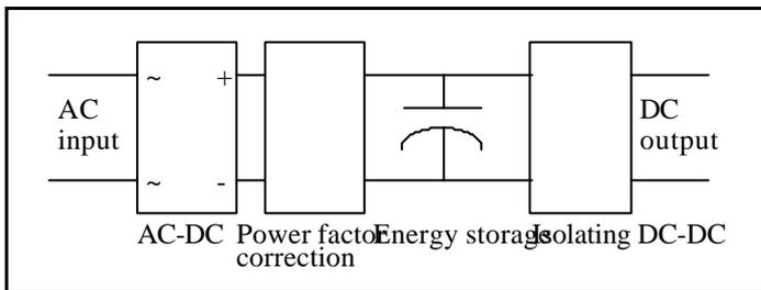
Fig 1. Block diagram of rectifier
