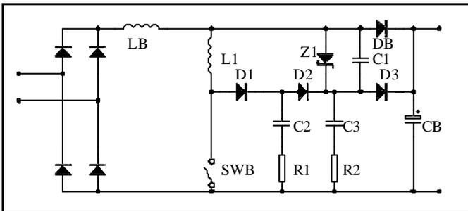
Fig 8. Circuit of Fig 6 with enhancements to new snubber.
