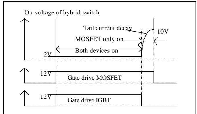
Fig 5. Idealised waveforms of the hybrid switch
