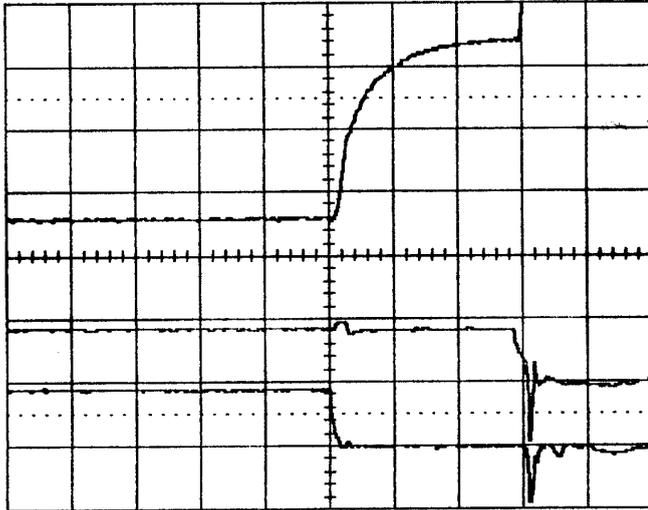
Fig 11. Observed hybrid switch performance in Boost stage. Top trace:  $V_{on}$  @2V/div, centre line is 0V; Lower traces: gate voltages on MOSFET and IGBT @10V/div; 0.5μsec/div horizontal.
