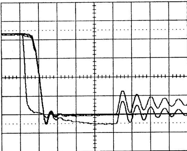
Fig 12. Observed lossless snubber operation at turn-on. 100V/div, 200nsec/div
