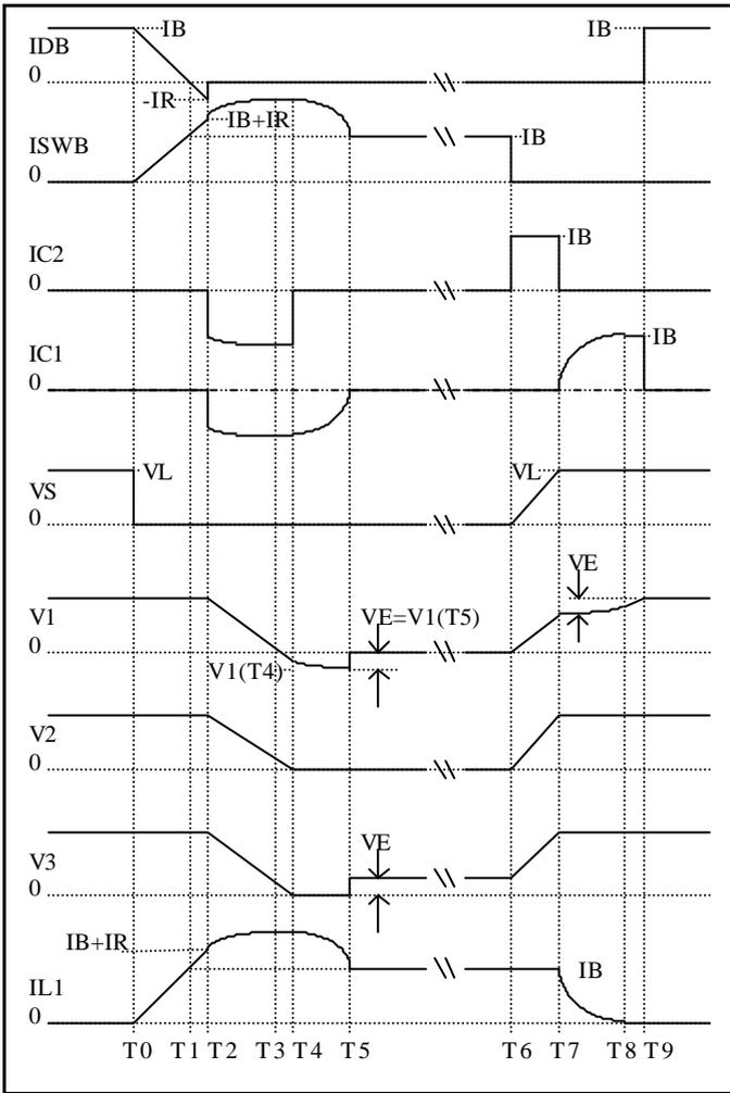
Fig. 7 shows the various waveforms at different parts of a switching cycle.
