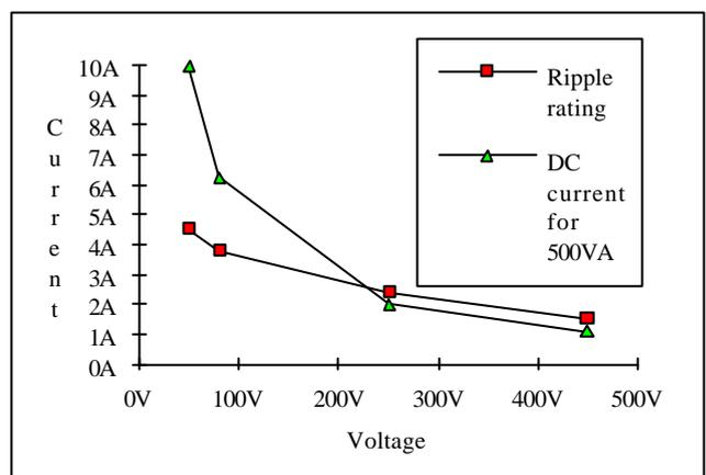
Fig 2. Ripple rating vs. voltage rating for capacitors of the same
