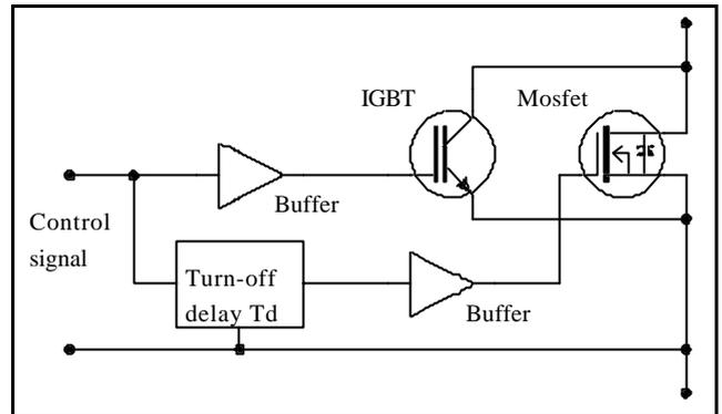
Fig 4. Schematic of the hybrid switch
