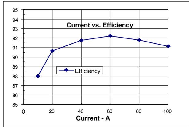
Fig. 2 Efficiency of 100A Rectifier
