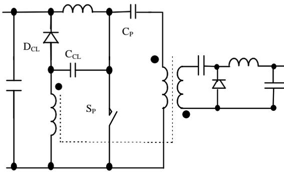
**Fig 6.** Cuk converter with clamp.
