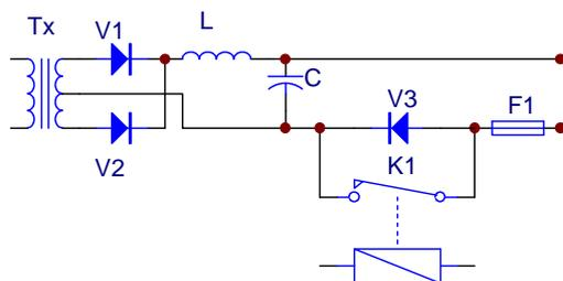
**Fig 1.** Proposed power circuit.
