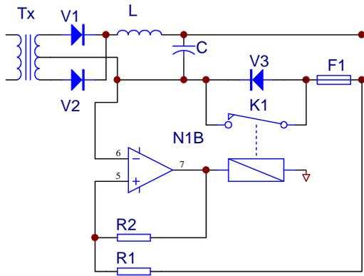
**Fig 2.** Simplified control circuit.
