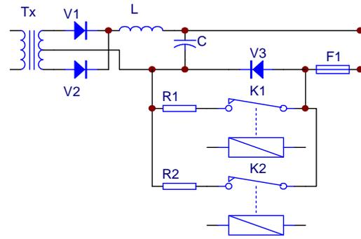
**Fig 3.** Arrangement for paralleling relays.
